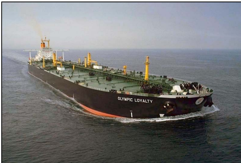
Figure 1-3 Typical VLCC-Class Tanker 303,000 DWT Olympic Loyalty
