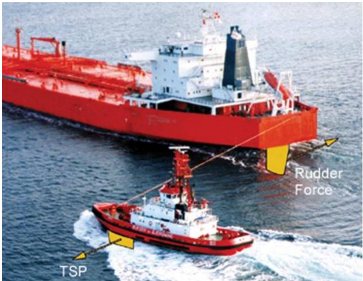
Fig A.1 Example of a Voith Schneider escort tug assisting a large tanker. TSP (Tons SteeringPull)
