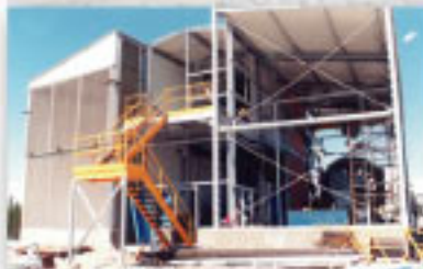
800,000 SCFM Direct Fired, Horizontal Discharge Mine Air Heater - Propane
