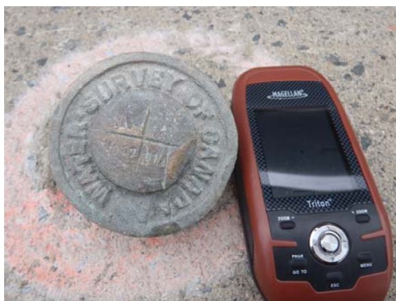
Picture 30: Damaged WSC benchmark.
