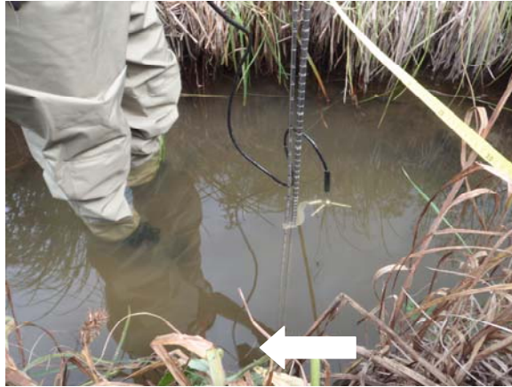
Picture 8: Flow Measurement taken across 1.3 m cross section.
