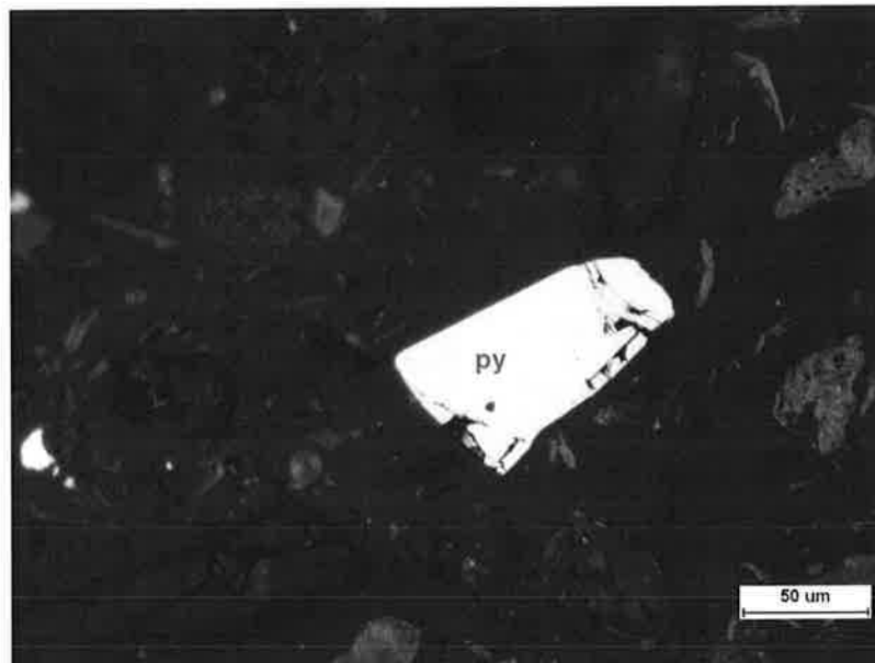
Figure 21. Liberated Pyrite in 2010-HR-091 PPRL photomicrograph of a liberated particle of pyrite.
