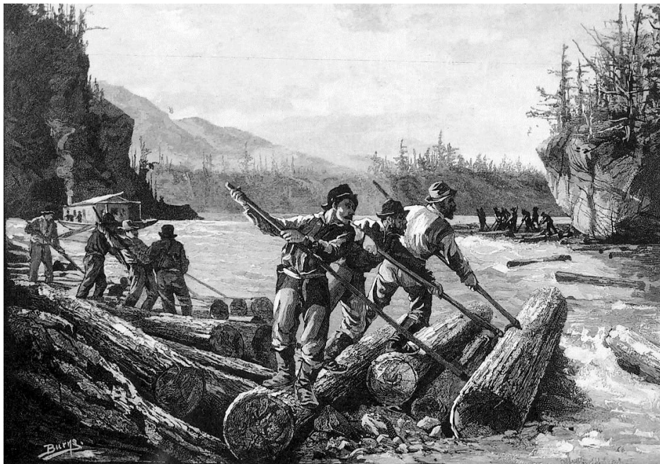
Photo 6.2.3 The drive, ca. late 1800s. Photographer, lithographer, and artist unknown. Loggers holding peavies are attempting to roll logs into the water. P4-3-12 New Brunswick Museum photographs collection, Provincial Archives of New Brunswick (PANB n.d.).
