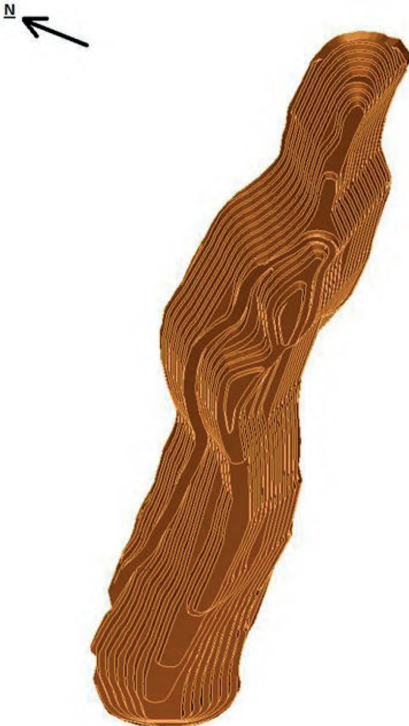
Figure 4.4 Final 3D Southwest Pit Design
