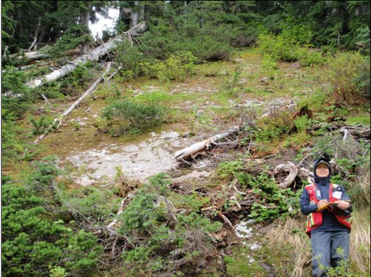
Photograph 23 North Treaty Upper Access Road – Looking upslope approximately 15 m from Km 2+400 of the North Treaty Upper access road towards a bedrock exposure. The bedrock is a slightly weathered (W2), medium strong (R3) sandstone with a highly persistent joint set that strikes sub parallel to the proposed road centerline (dip/dip direction is 44/043 degrees with joint persistence >18 m).
