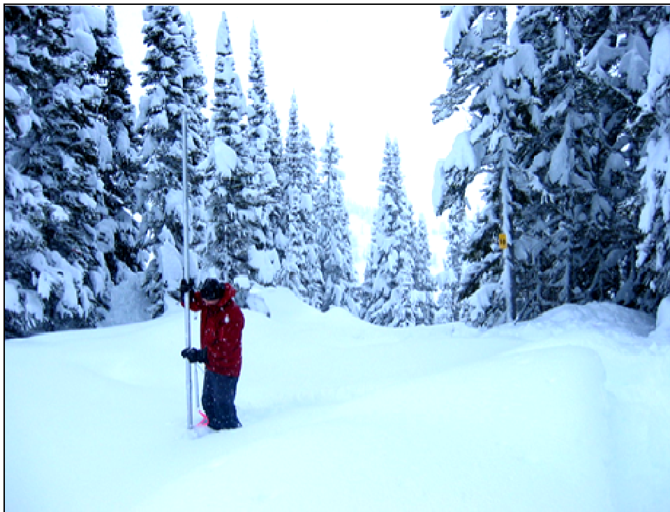
Plate 2.6-1. A snow core being collected using a Standard Federal Snow Sampling Kit. This is the equipment that is recommended in the BC MOE Snow Survey Sampling Guide (BC MOE 1981) and was used at KSM.
