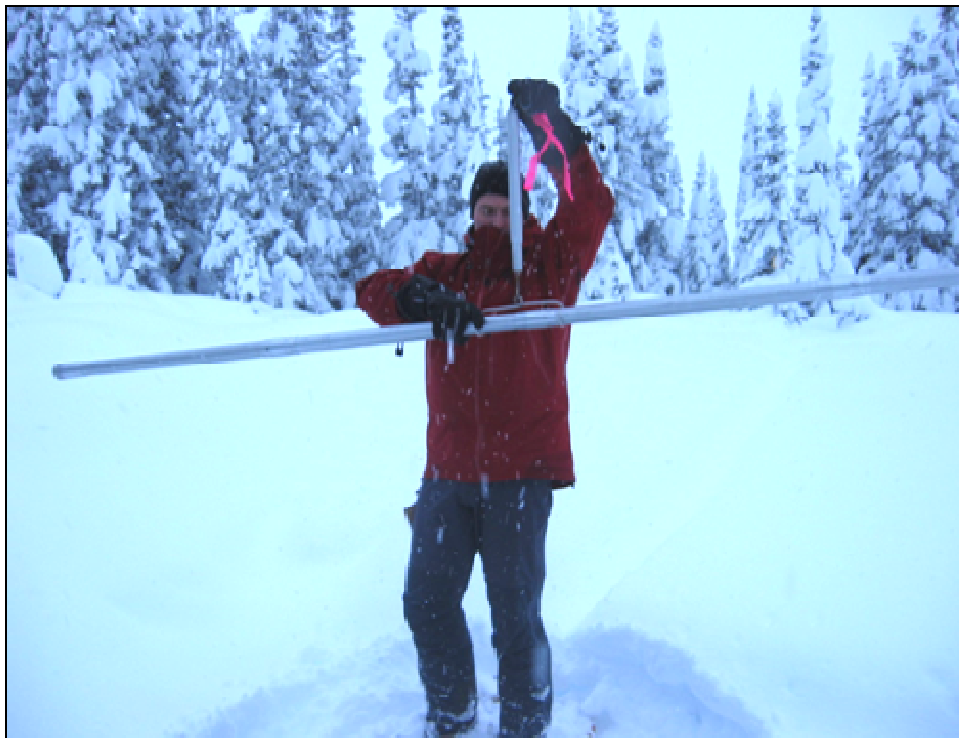
Plate 2.6-2. A snow core being weighed using a calibrated spring scale to determine SWE.
