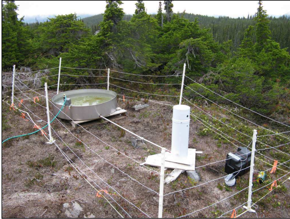
Plate 2.5-1. Teigen Evaporation Pan (July 2011).
