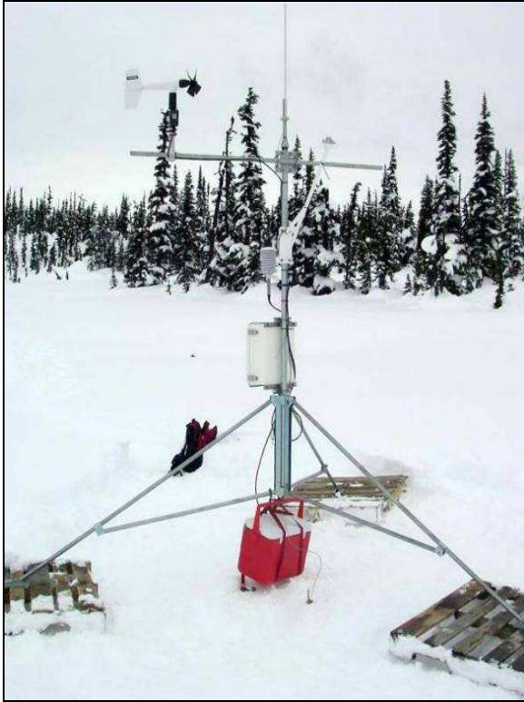
Plate 2.2-2. Teigen Creek temporary tripod meteorological station (March 2008).
