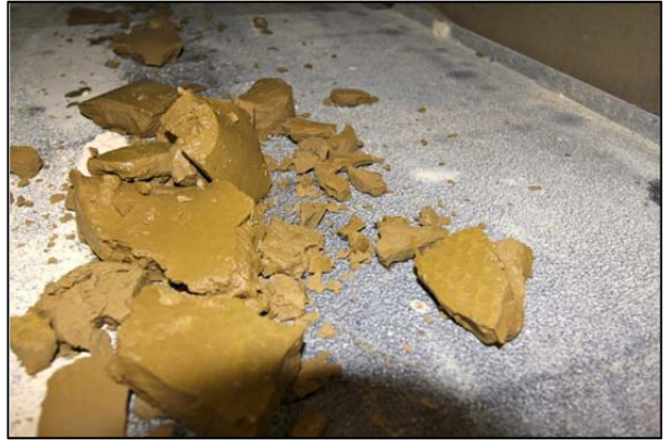
Sludge Filter Cake: 40% Moisture
