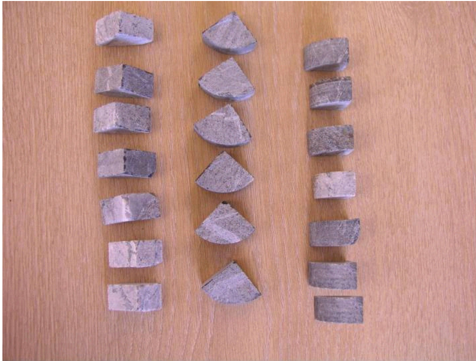
Figure 3 – Orientations of Pieces for Breakage (Cut Core Method)
