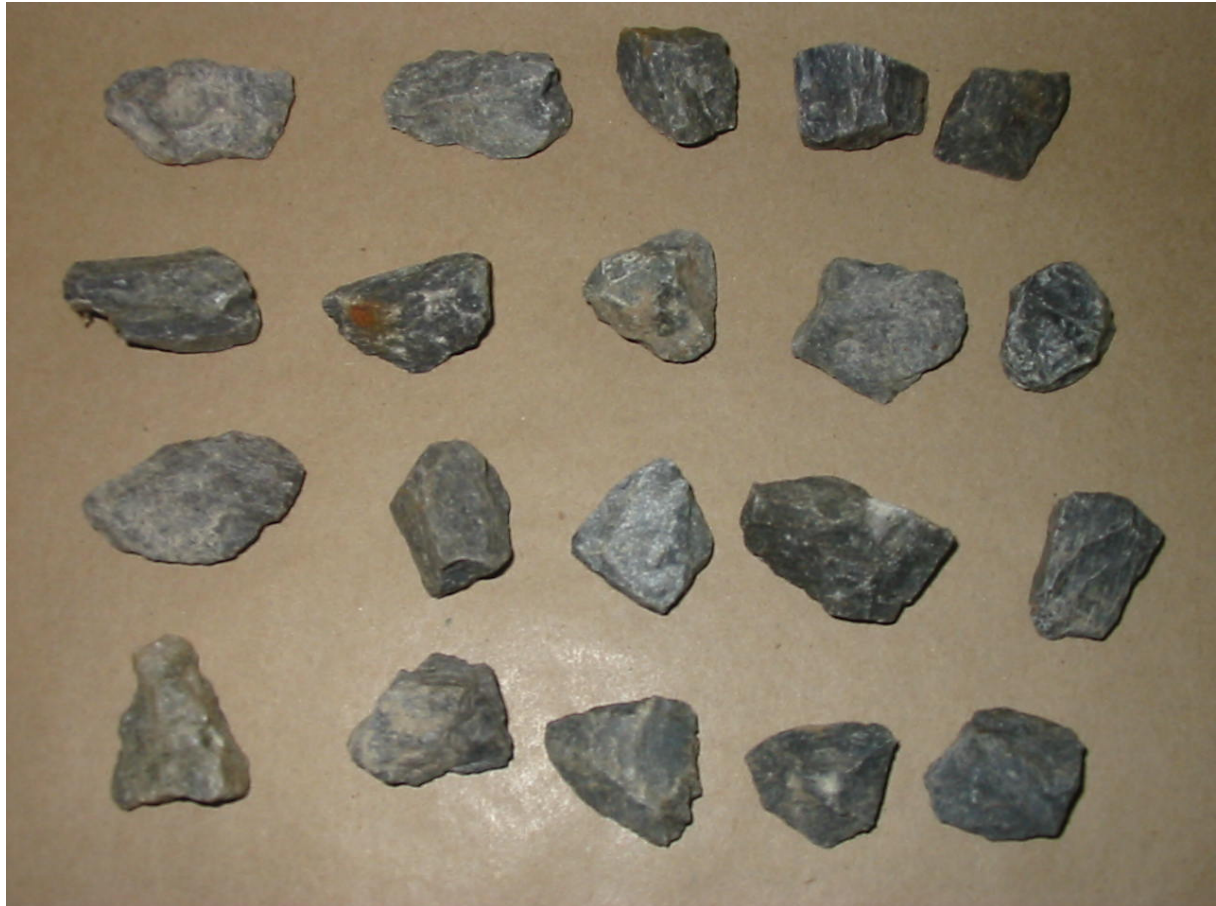
Figure 2 – A Typical Set of Particles for Breakage (Particle Selection Method)
