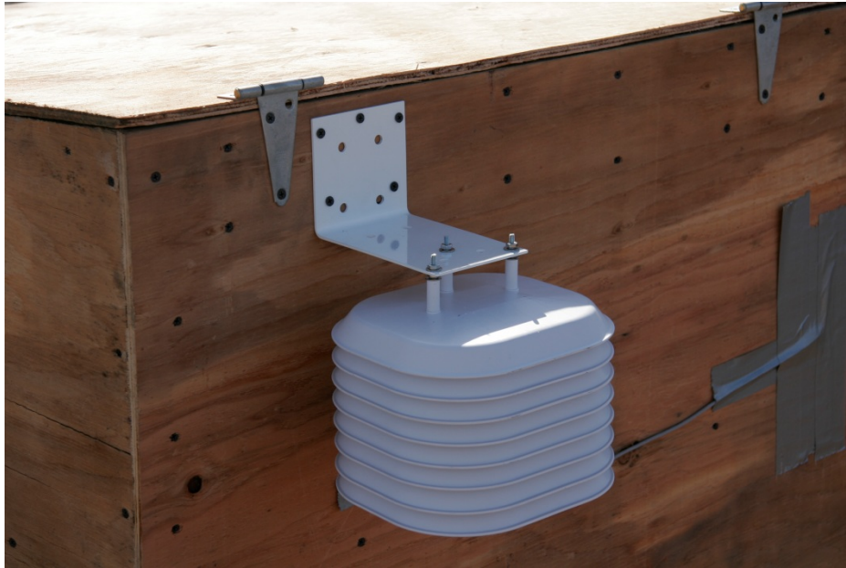
Photo 3: Air Temperature Sensor attached to outside of housing.
