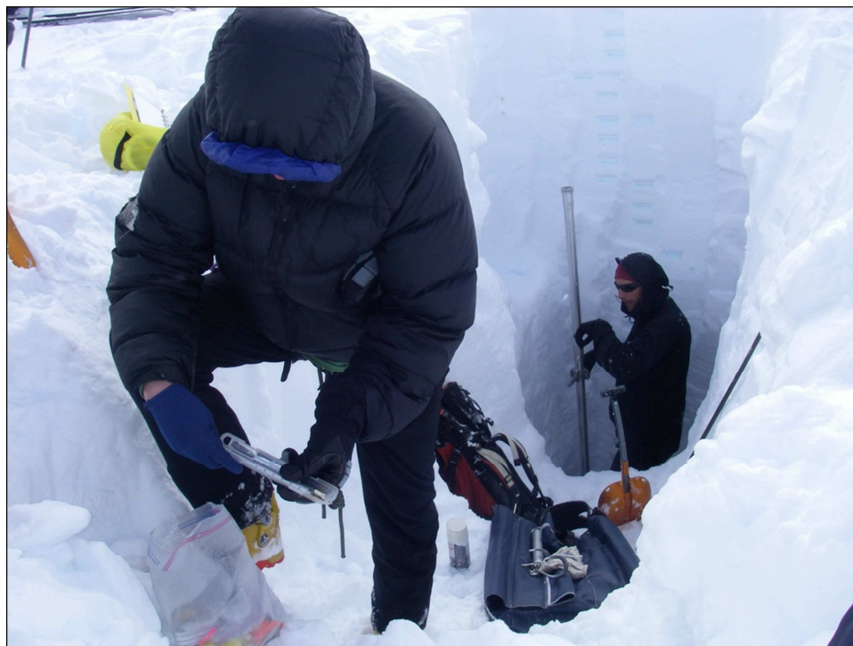
Plate 3.2-1. Measuring snow density at McTagg West Glacier (1,700 masl) in April 2011.
