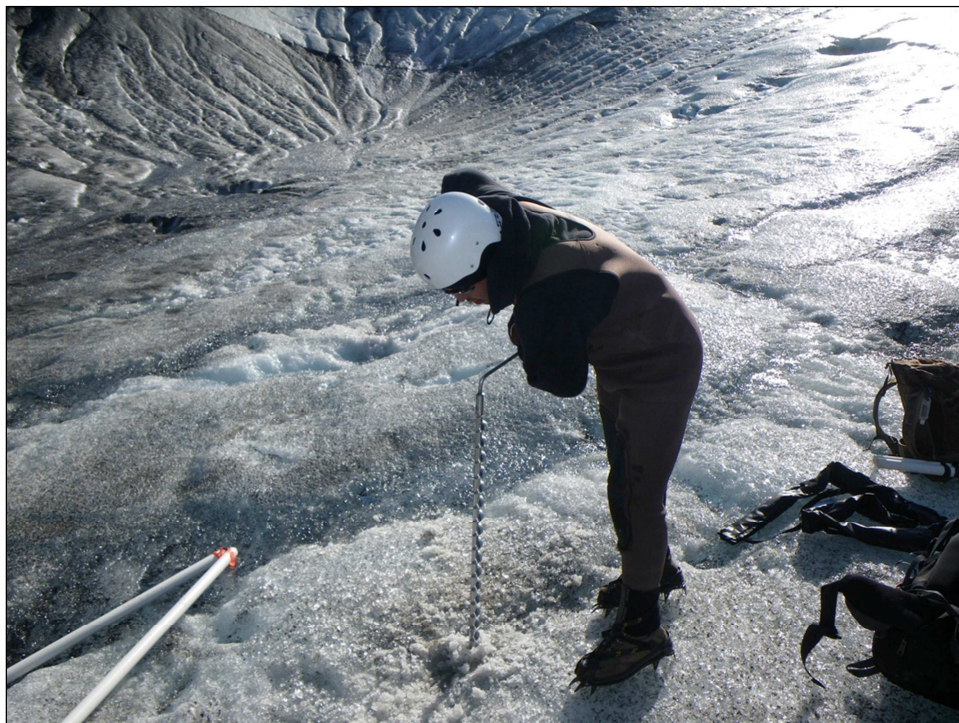
Plate 3.2-4. Ablation stake, MI-900 being redrilled level with the ice surface in August 2011.
