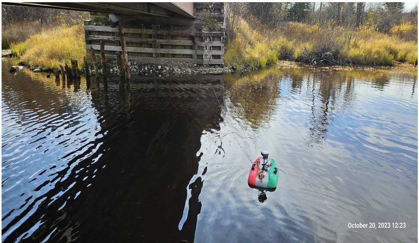
Photo 10. Reach 1 - Facing north – hydrology surveying unit measuring flow. October 20, 2023
