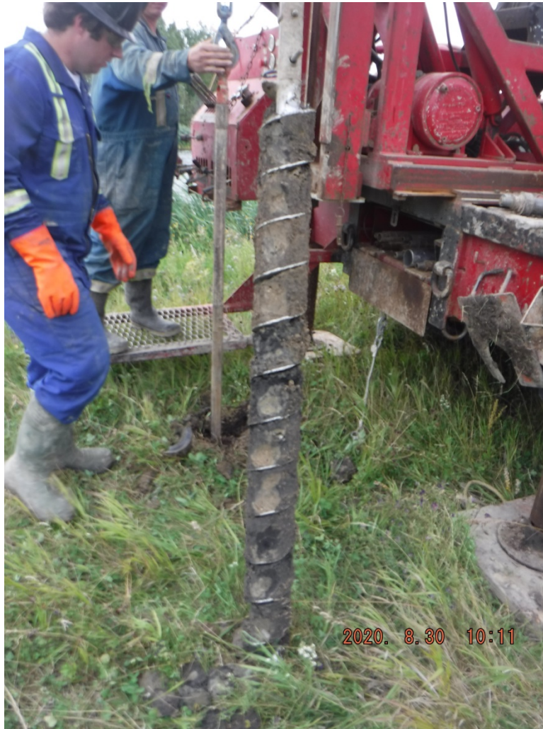
Photograph 5: Buried organics in BH20-B02 (existing berms)
