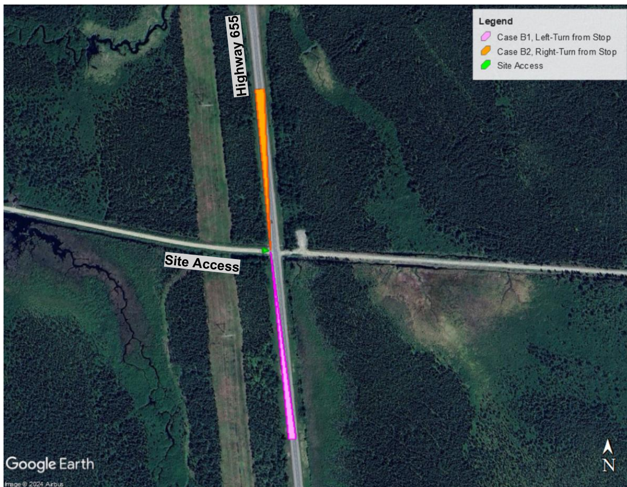
Figure 5.1 Intersection Sight Distance Requirements for Left/Right Turns Out of the Existing Project Access
