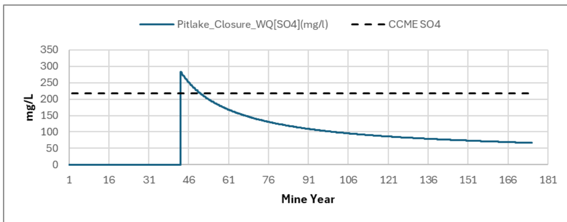
Figure D.1.6-1: Water quality model results for SO 4 at Pit Closure.
