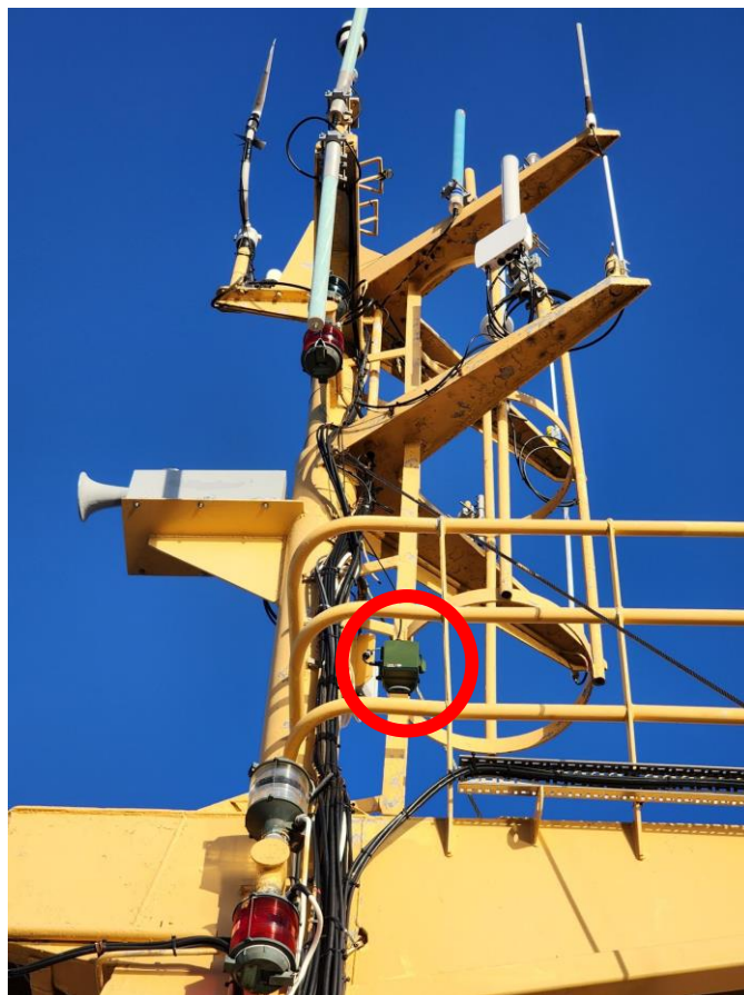
Figure 2: Vessel-mounted Autonomous Recording Unit and Ultrasonic Microphone.
