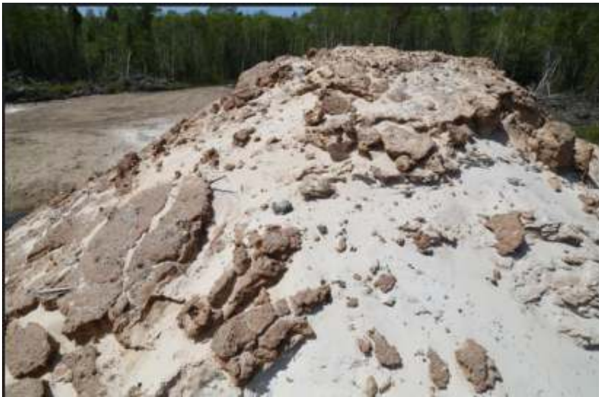
Figure 3. Concretions potentially containing sulphide in pyrite and marcasite in sand piles extracted near Vivian Manitoba in the spring of 2020.
