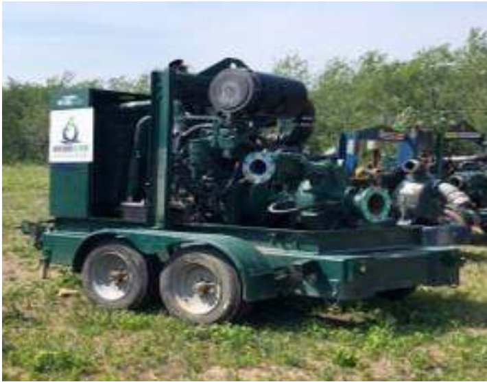
Figure 26. Compressor used by CanWhite to inject air for sand extraction from the Winnipeg Formation aquifer
