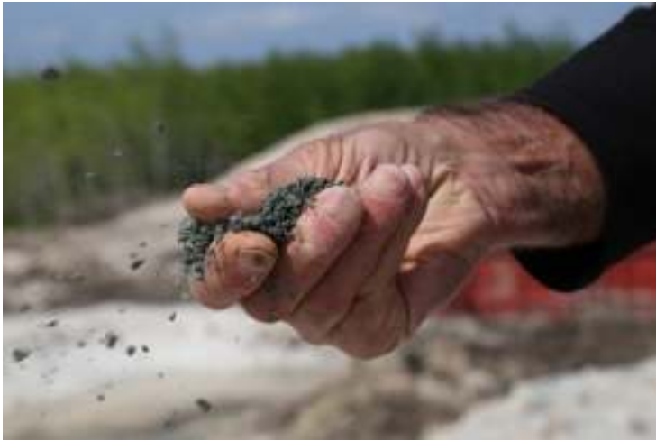
Figure 15. Fragility of shale brought to the surface by solution mining sand extraction from about 200 feet below the surface near Vivian.
