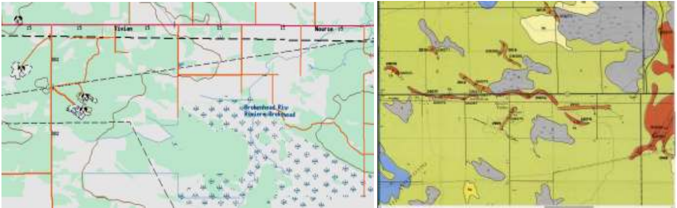
Figure 14 a and b. Topographical map (a) of Vivian area and surface composition map (b) showing the natural drainage path to the Brokenhead River. Sand and gravel deposits are shown in brown in the drainage path to from the Vivian plant site area to the Brokenhead River.
