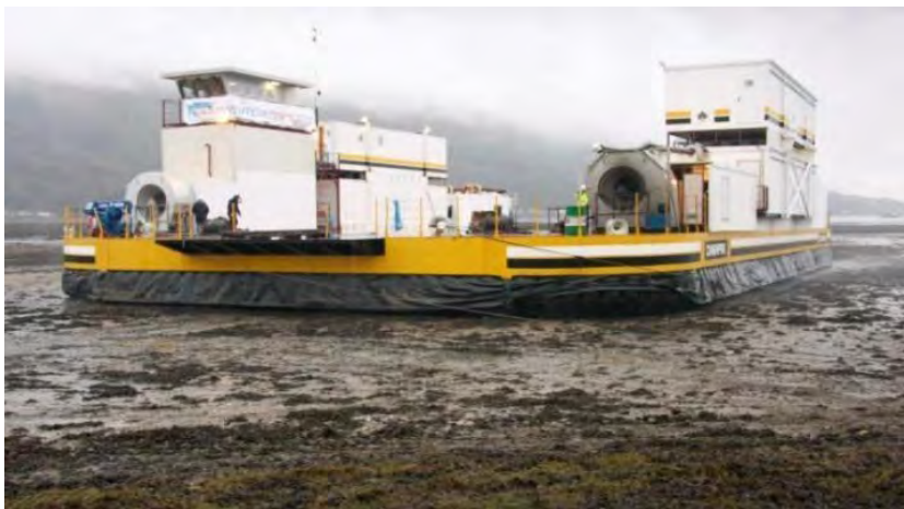
Figure 3.1: 200t Cold Weather Heavy Lift Hoverbarge (2009)
