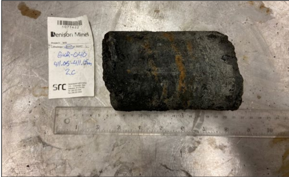
Figure F-3: Coreflood 4 Feed Sample Side View, Prior to Placement in Coreflood Machine
