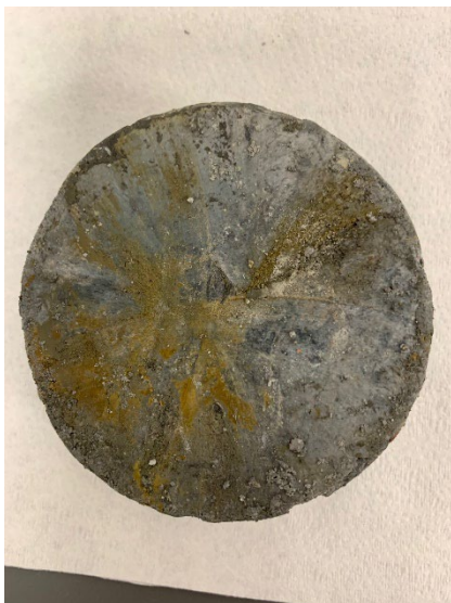
Figure F-7: Coreflood 4 Discharge End Puck (Section 1), Inlet Face View, Dried
