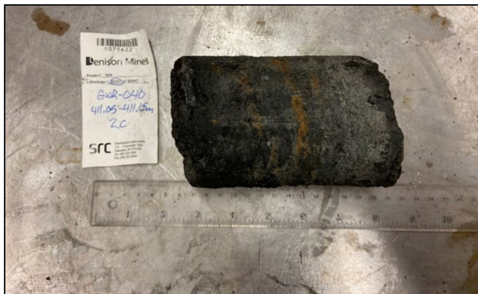
Figure 3: Coreflood 4 Feed Sample Side View, Prior to Placement in Coreflood Machine
