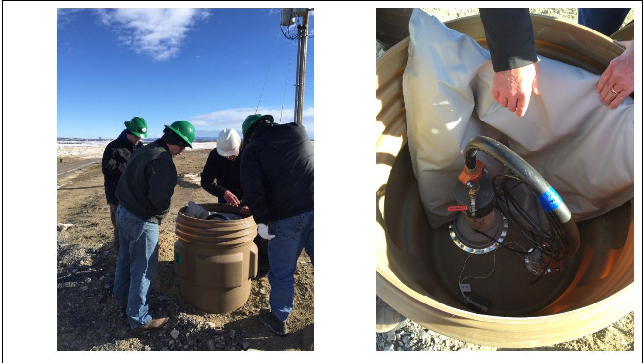
Figure 2.9: Typical In Situ Recovery Well at Surface
