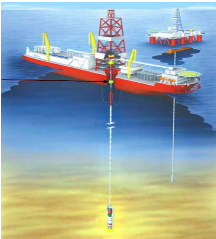
Figure 2-2 Illustration of Drill Ship (front) and Semi-submersible (back)
