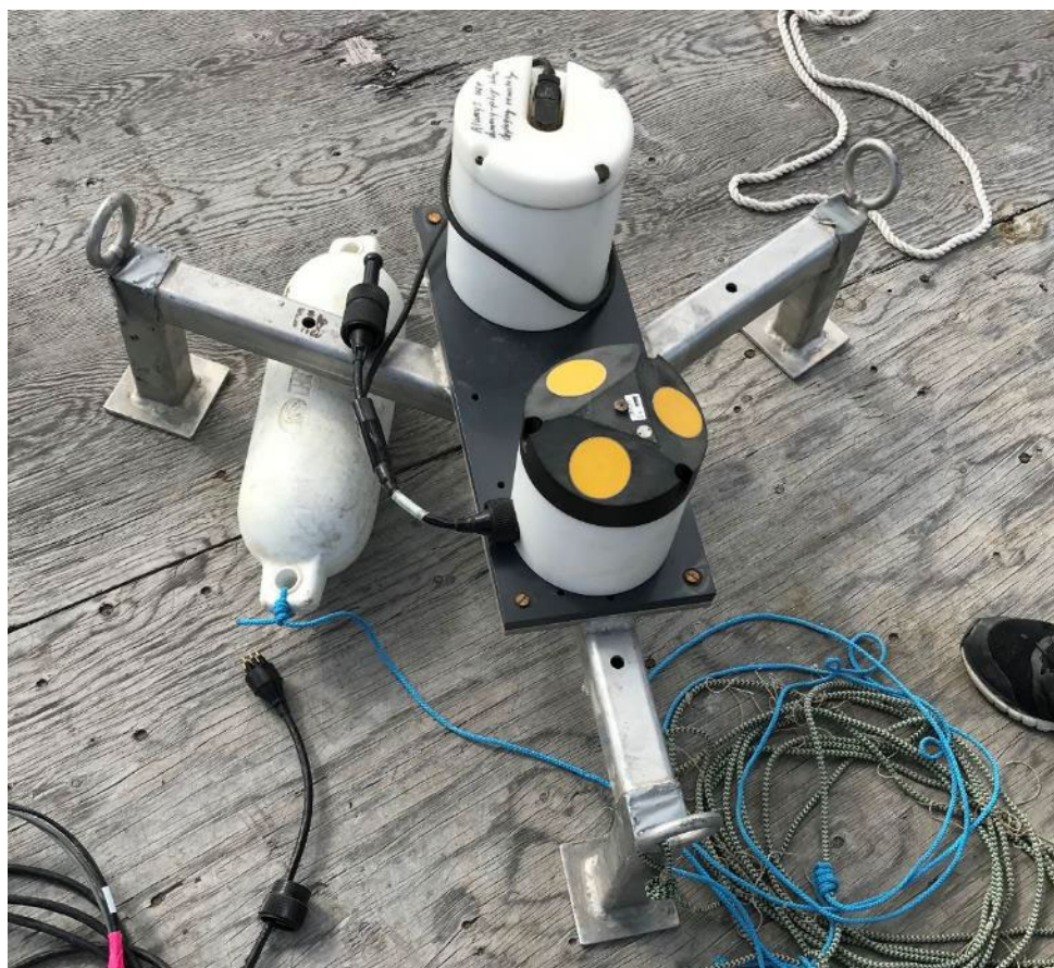
Figure 7: Sontek Argonaut-XR Acoustic Doppler Current Profiler and Mounting Frame Deployed at Patterson Lake South
