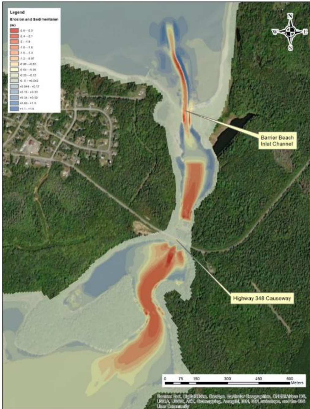
Figure 8: Cumulative Erosion and Sedimentation One Year Following Dam Removal
