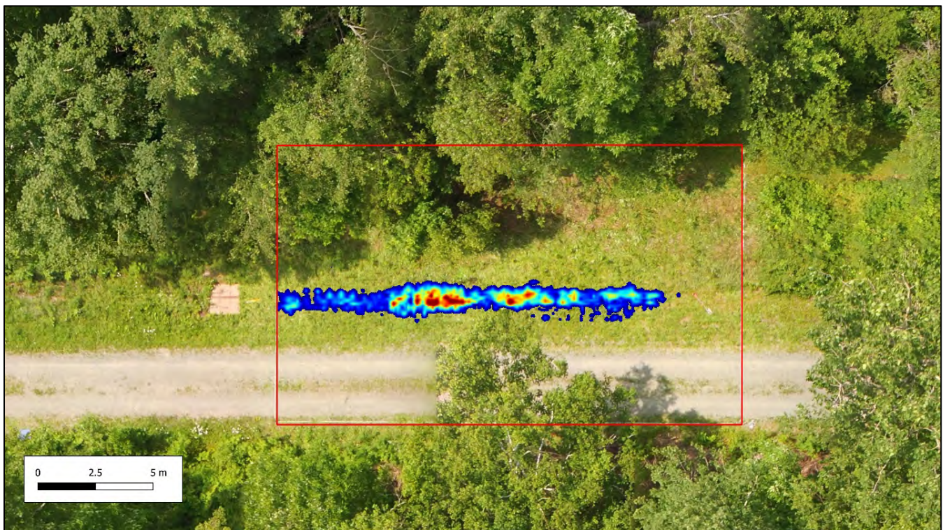
Plate 12: Pipeline response isolated.
