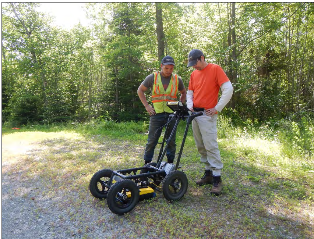
Plate 2: Preparing the Noggin 500 GPR for survey along the existing pipeline.
