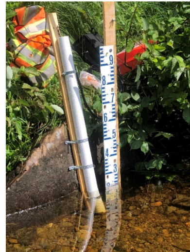
Photo 4: Hydrometric Station Installed at SW14
