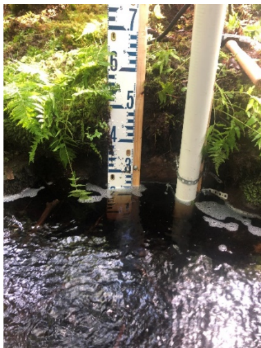
Photo 5: Hydrometric Station Installed at SW15
