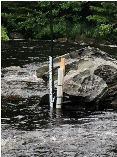
Photo 3: Hydrometric Station Installed at SW6
