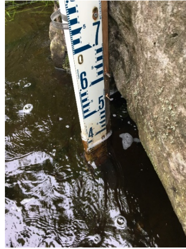
Photo 2: Hydrometric Station Installed at SW5
