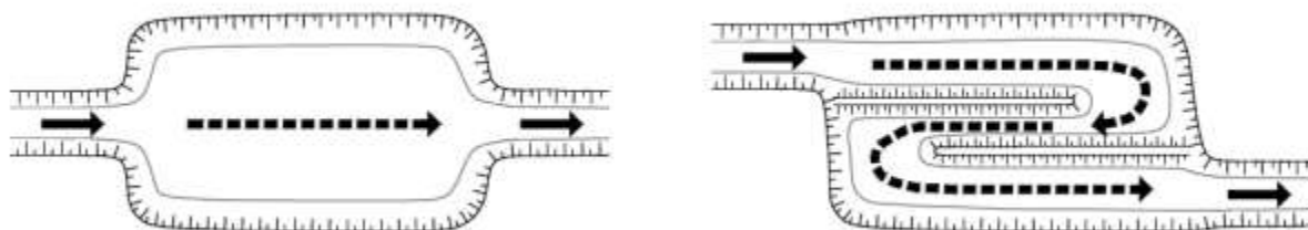
Figure 4: Flow Plath Lengths in Settling Basins
