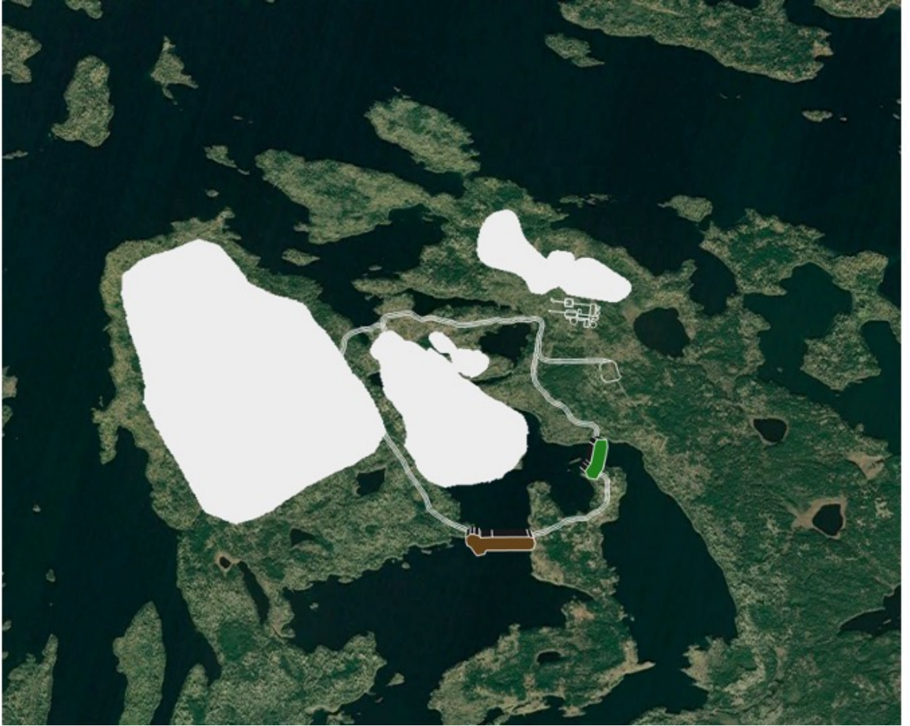
Map 3: Proposed layout of the Springpole Gold Project. The white polygons represent, from left to right, mine rock storage, open pit and stockpiles, process plant and waste rock storage. The map also shows the location of two coffer dams (brown and green), and mine road (source: First Mining Gold).
