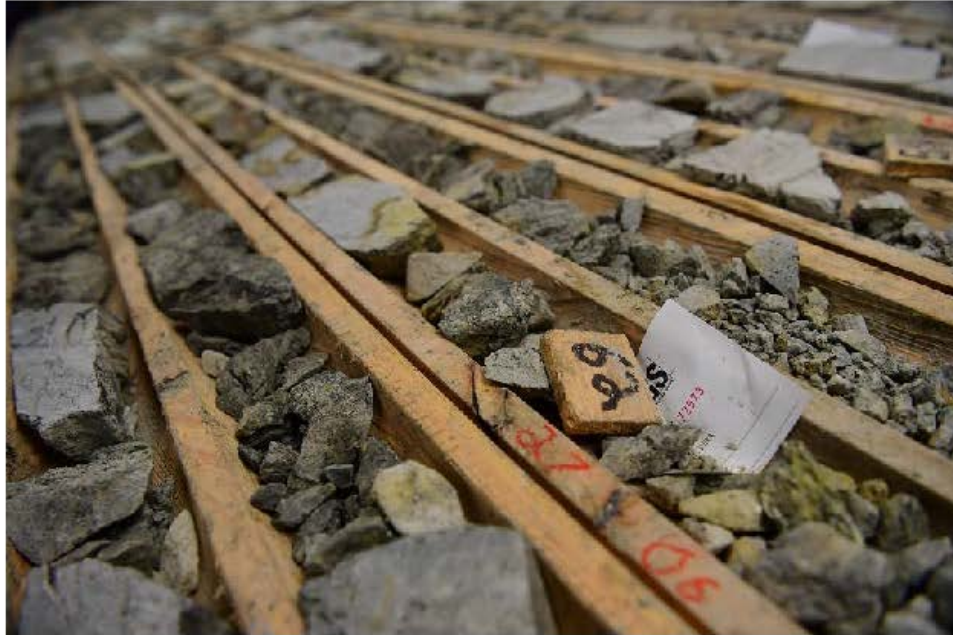
Figure 4: Photo of mineralized core from the Portage zone showing the extreme friability of the potassic-altered rock.
