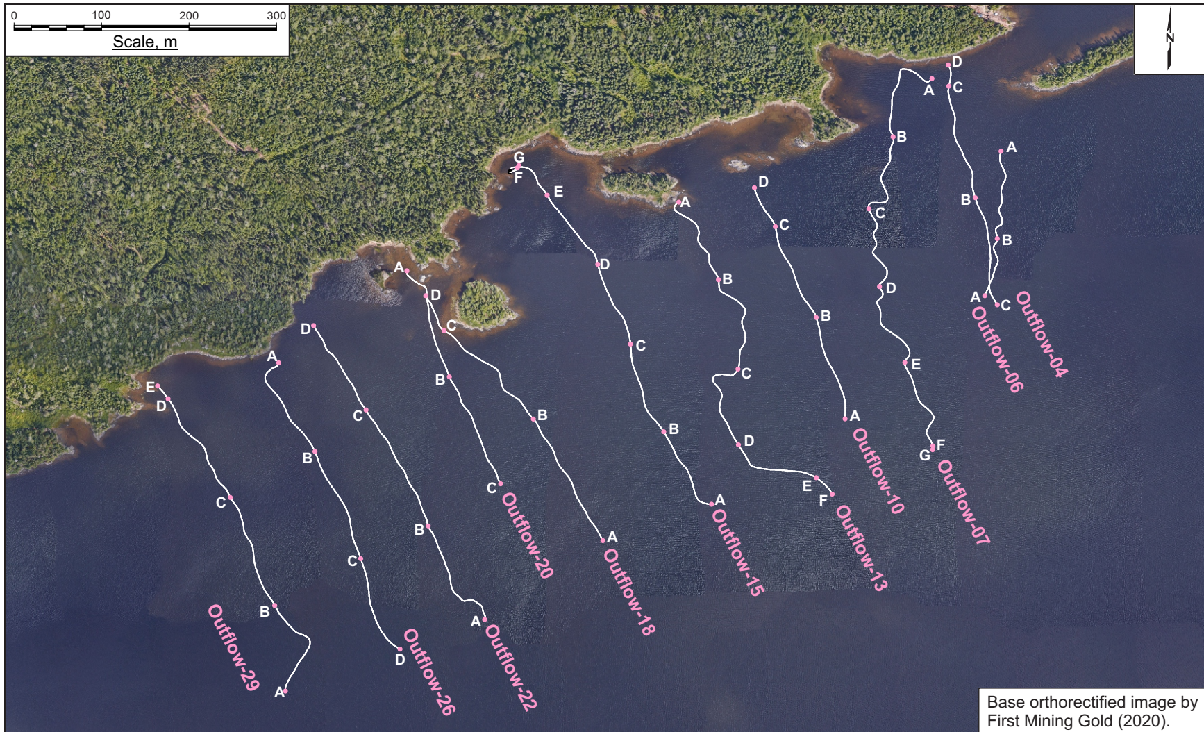
Figure E20 Location of the GPR survey conducted on the water (lake) surface along the proposed Outflow area in August 2020.
