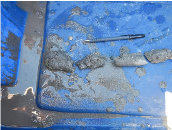
Photo ID: DSCN 3748 Dominant material: Fine sand and silt Secondary material: Fine gravel Top size: 1 cm Description: Material extracted from bed shown in a pail. Pen for scale points to the top of the core.
