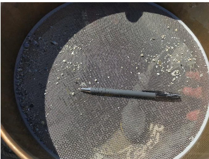
Photo ID: IMG 0525 Dominant material: Fine sand and silt Secondary material: Shells in thin upper silty layer Top size: N/A Description: Material extracted from bed shown washed through a 1.18 mm sieve plate.
