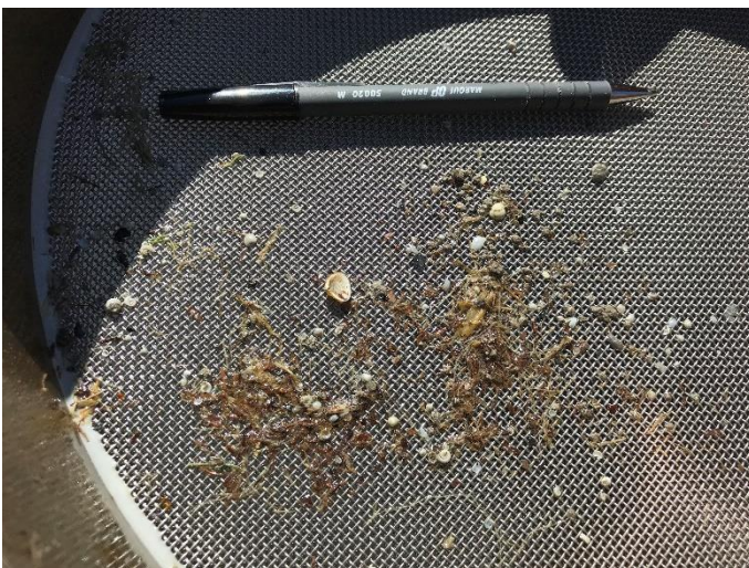
Photo ID: IMG 0533 Dominant material: Fine sand and silt Secondary material: N/A Top size: N/A Description: Material extracted from bed shown washed through a 1.18 mm sieve plate.
