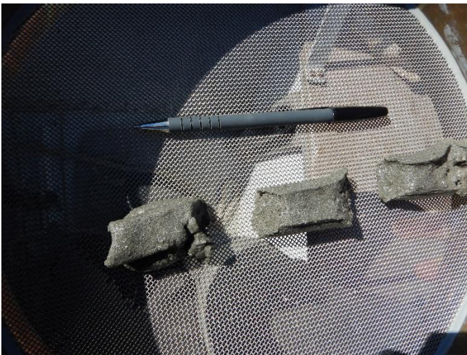
Photo ID: DSCN 3752 Dominant material: Fine sand and silt Secondary material: N/A Top size: 3 mm Description: Material extracted from bed shown on a sieve plate. Pen for scale points to the top of the core.
