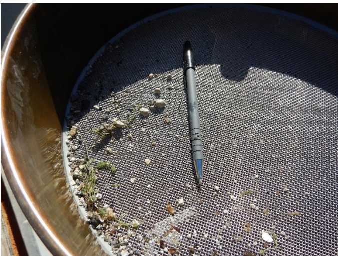
Photo ID: DSCN 3749 Dominant material: Fine sand and silt Secondary material: Fine gravel Top size: 1 cm Description: Material extracted from bed shown washed through a 1.18 mm sieve plate.
