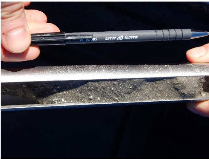
Photo ID: DSCN 3761 Dominant material: Fine sand and silt Secondary material: N/A Top size: 5 mm Description: Material extracted from bed using hand auger.
