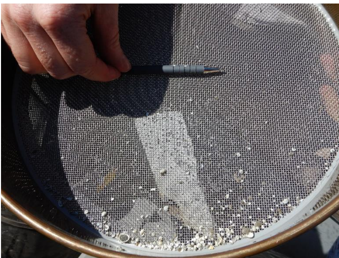
Photo ID: DSCN 3763 Dominant material: Fine sand and silt Secondary material: N/A Top size: 5 mm Description: Material extracted from bed shown washed through a 1.18 mm sieve plate.
