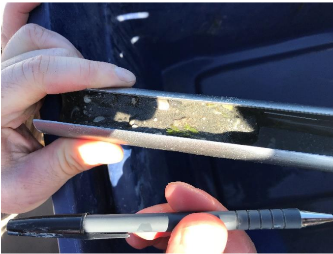
Photo ID: IMG 0527 Dominant material: Gravelly sand Secondary material: N/A Top size: 2.5 cm Description: Material extracted from bed using hand auger.
