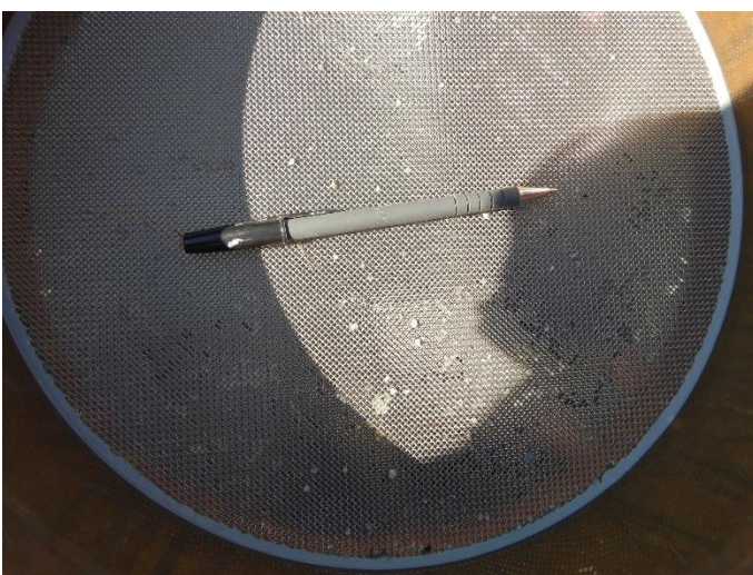
Photo ID: DSCN 3753 Dominant material: Fine sand and silt Secondary material: N/A Top size: 3 mm Description: Material extracted from bed shown washed through a 1.18 mm sieve plate.
