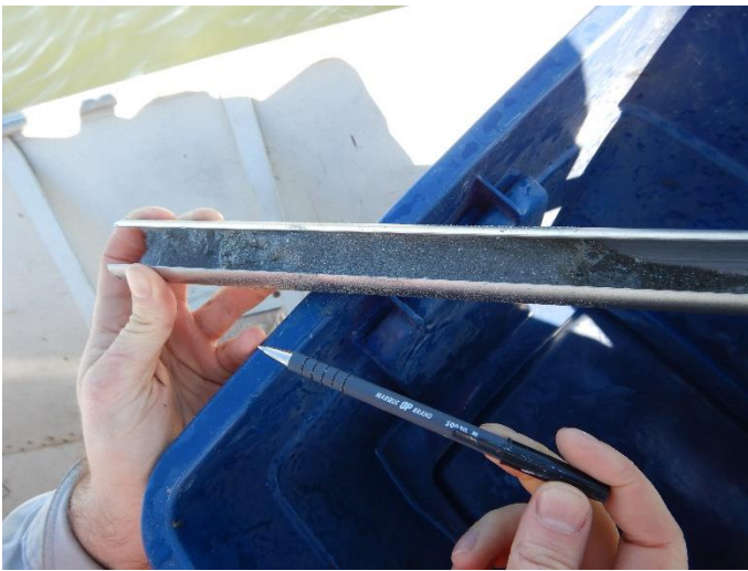
Photo ID: DSCN 3751 Dominant material: Fine sand and silt Secondary material: N/A Top size: 3 mm Description: Material extracted from bed using hand auger.
