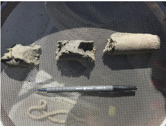
Photo ID: IMG 0532 Dominant material: Fine sand and silt Secondary material: N/A Top size: N/A Description: Material extracted from bed shown on a sieve plate. Pen for scale points to the top of the core.
