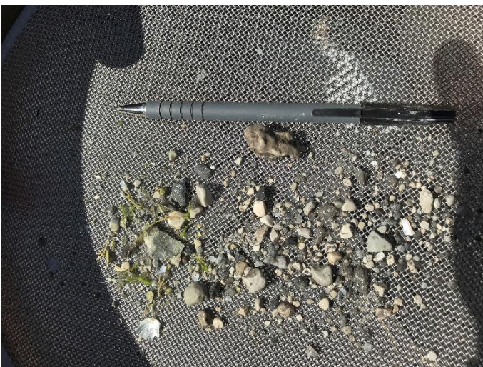
Photo ID: IMG 0529 Dominant material: Gravelly sand Secondary material: N/A Top size: 2.5 cm Description: Material extracted from bed shown washed through a 1.18 mm sieve plate.
