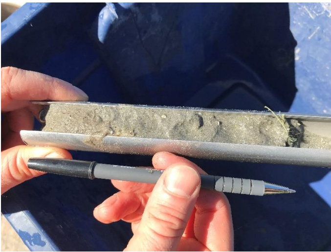
Photo ID: IMG 0531 Dominant material: Fine sand and silt Secondary material: N/A Top size: N/A Description: Material extracted from bed using hand auger.
