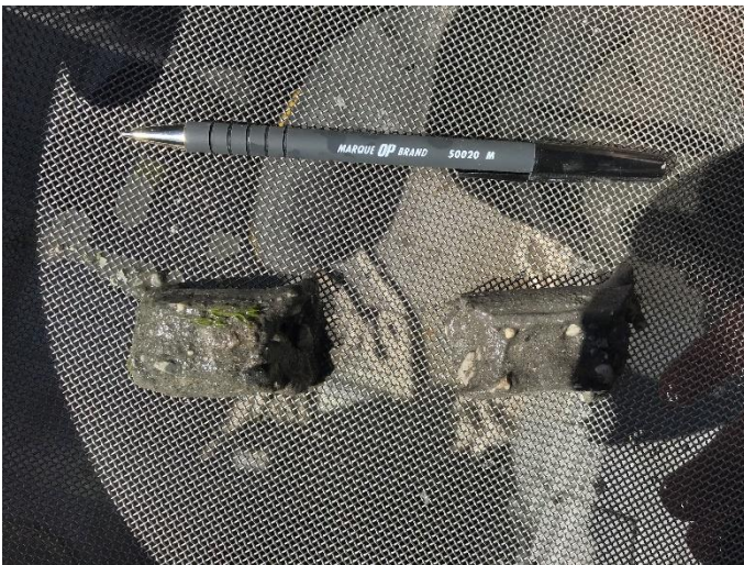
Photo ID: IMG 0528 Dominant material: Gravelly sand Secondary material: N/A Top size: 2.5 cm Description: Material extracted from bed shown on a sieve plate. Pen for scale points to the top of the core.
