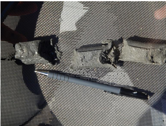
Photo ID: DSCN 3762 Dominant material: Fine sand and silt Secondary material: N/A Top size: 5 mm Description: Material extracted from bed shown on a sieve plate. Pen for scale points to the top of the core.
