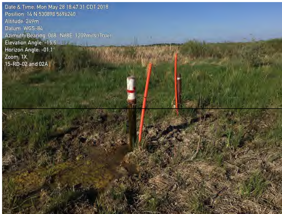
Figure 4: 15-RD-02, showing leaking casing and wet ground around well.
