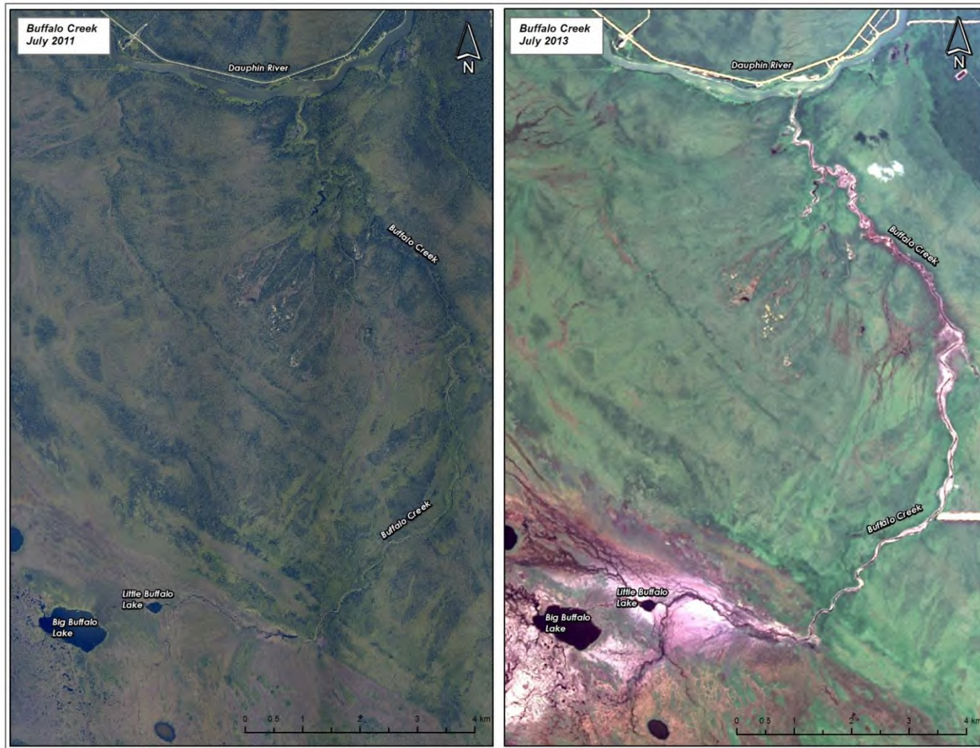
Figure 6.4-12. Satellite image overview of the Buffalo Creek watershed comparing Pre-Operation (July 2011) and 2011/2012 Closure (July 2013). Areas of bare soil resulting from flooding appear bright white, while light to dark brown areas are dead shrubs and trees.
