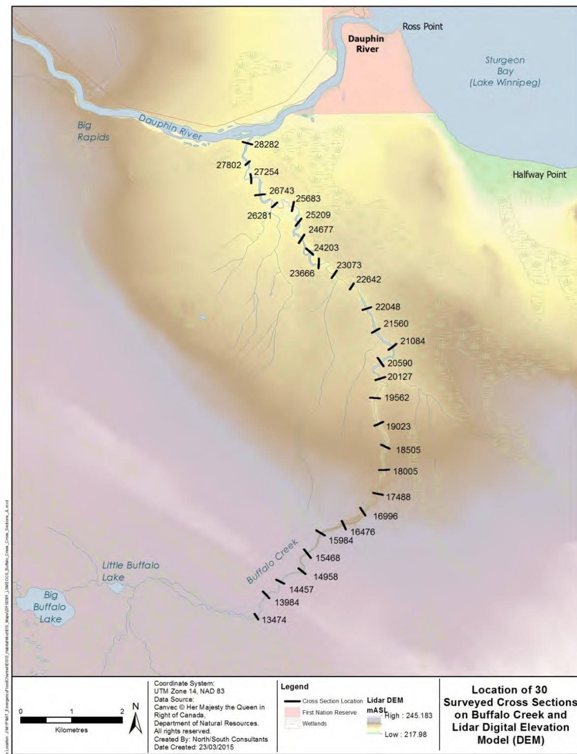
Figure 6.2-8. Map showing the location of the 30 surveyed cross sections along Buffalo Creek, the LiDAR based digital elevation model is shown in the background.
