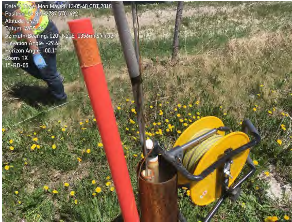
Figure 3: 15-RD-05, showing damaged lower standpipe. The foam insert could not be removed further due to damage to standpipe below.
