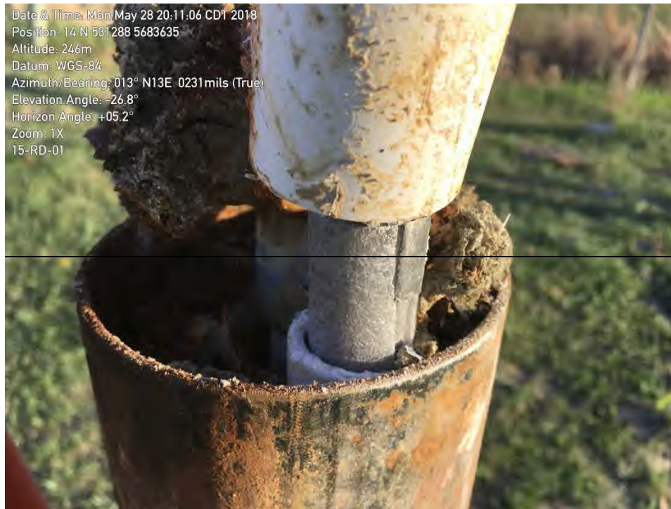
Figure 5: 15-RD-01, showing broken standpipe; obstruction also present at 1.497 m.
