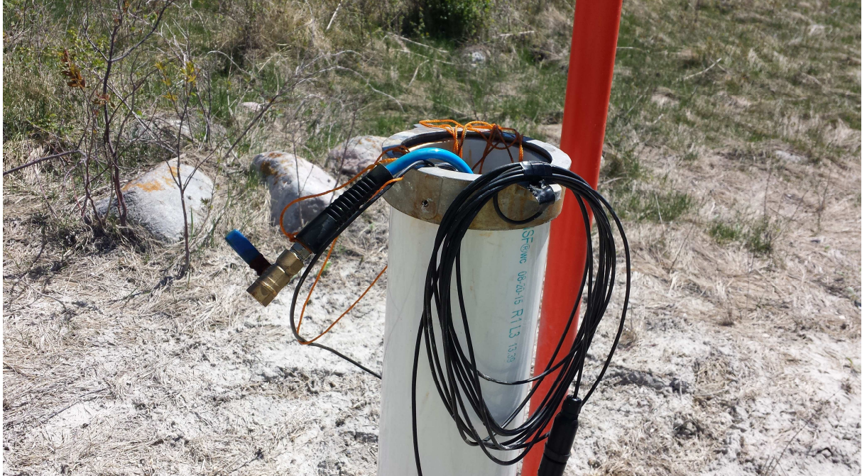
Photo 3. TH-ED-01 – Showing sample tubing and transducer port connection.
