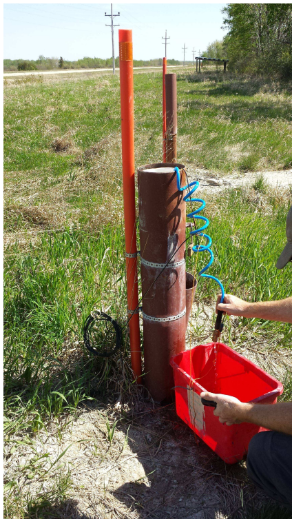
Photo 2. RD15-PW1 – Showing sample purging from tube.
