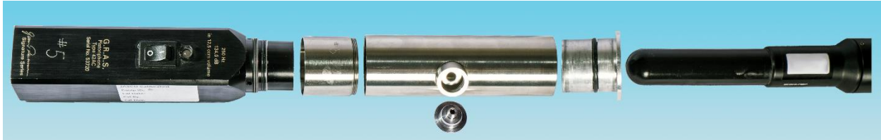
Figure C-8. Split view of a G.R.A.S. 42AC pistonphone calibrator with an M15B hydrophone.
