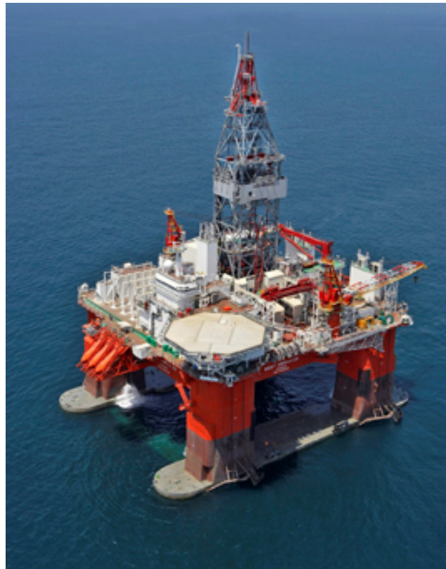
Figure 2-3 West Hercules – Example of a Semi-Submersible
