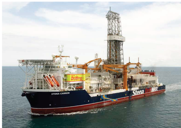
Figure 2-4 Stena Carron - Example of a Drill Ship
