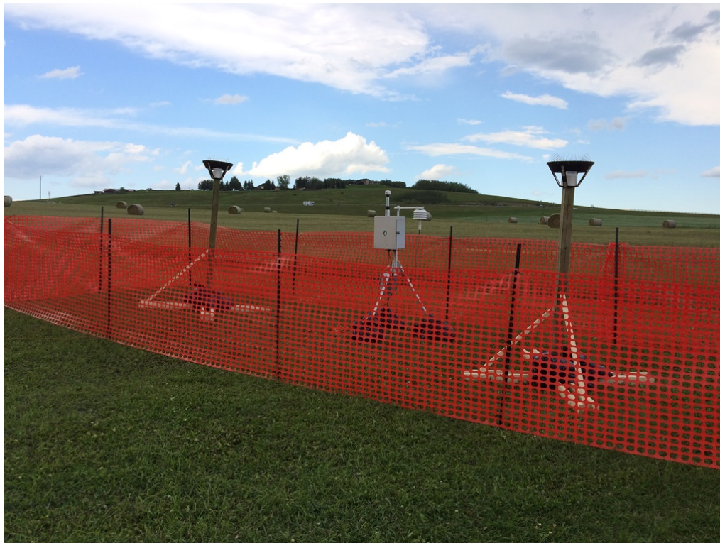
Photo 3D-1 EBAM Monitor (Centre) and Dustfall Collectors (Left and Right) at Parcel 56 on August 2, 2016 (Looking North). A Temporary Security Fence Was Used to Prevent Tampering or Vandalism.
