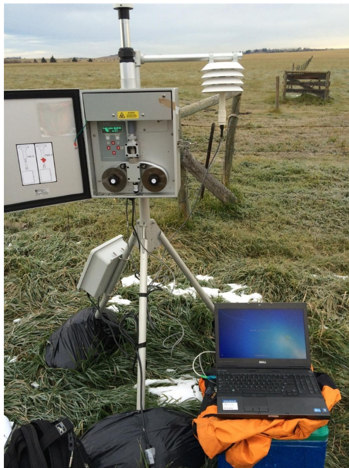
Photo 3D-5 Downloading PM 2.5 Data from EBAM Monitor to a Laptop Computer. October 13, 2016 (Looking North).
