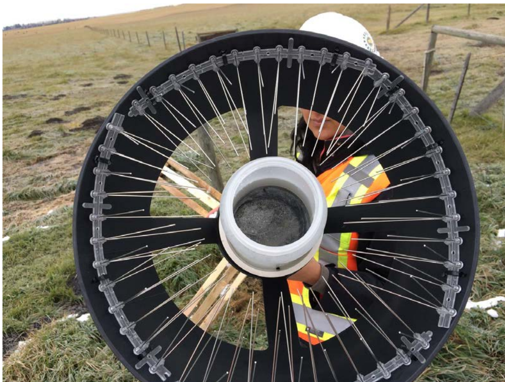
Photo 3D-6 Top View of Dustfall Collector Showing Wind Screen (Black), Bird Spikes and Sample Container (White). October 13, 2016.
