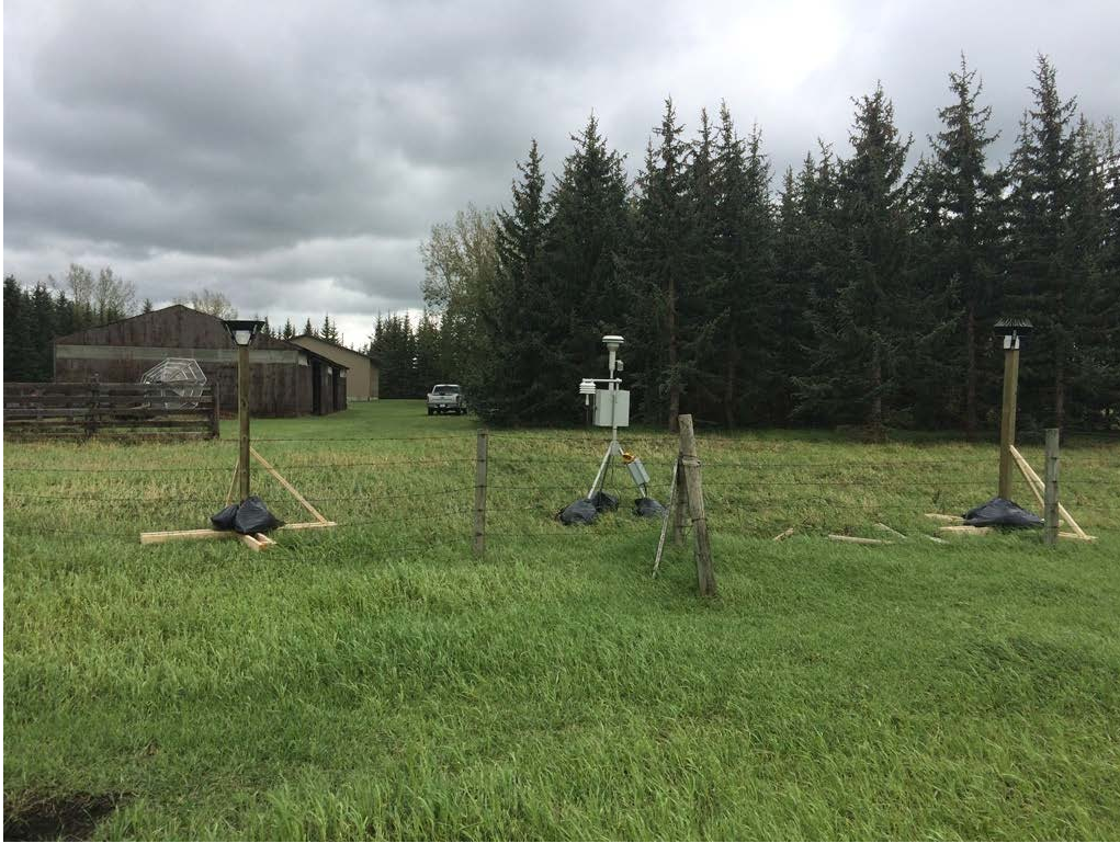
Parcel 58 – View South Toward E-BAM Particulate Monitors and dustfall collectors (August 3, 2016)
