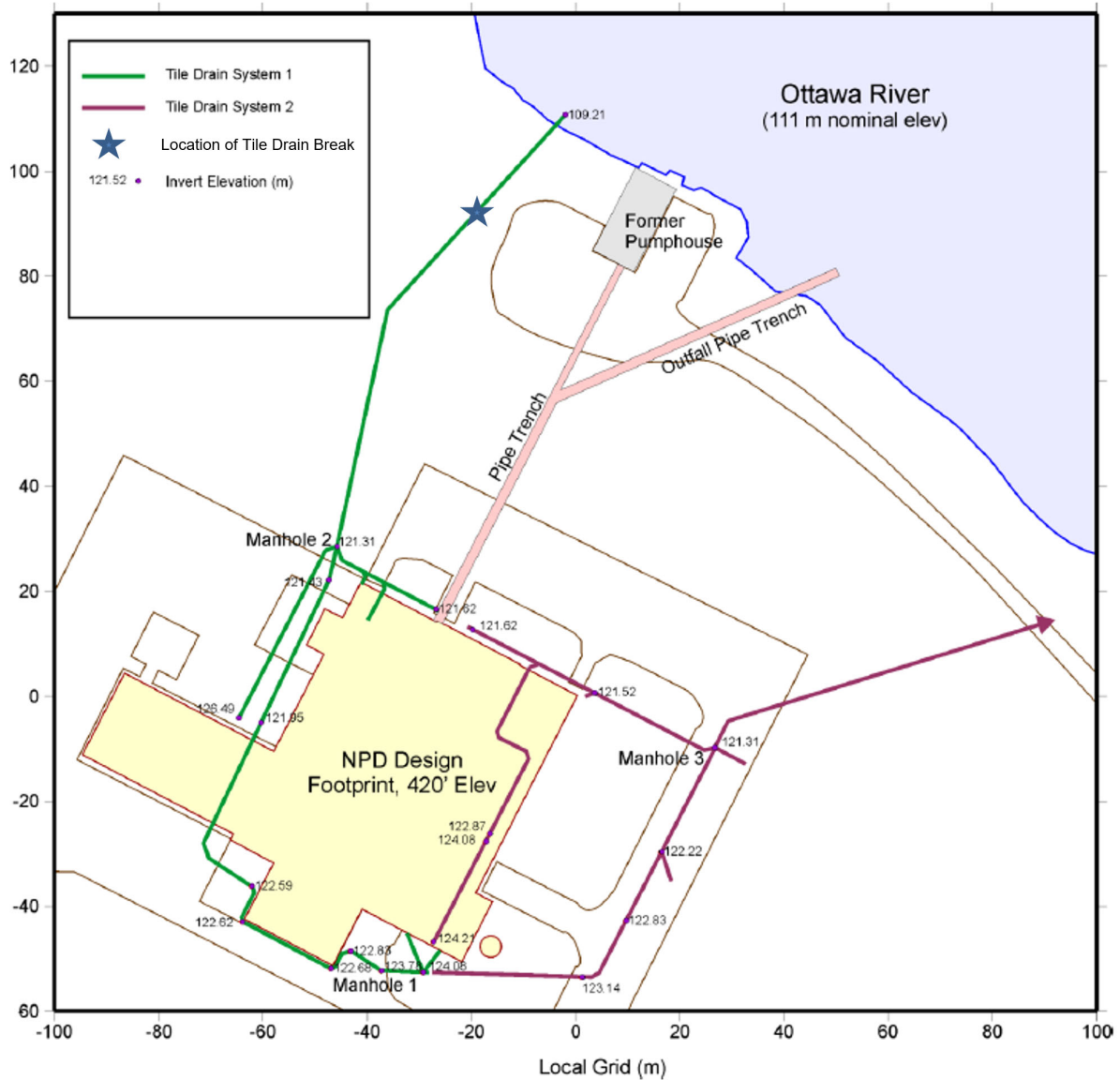
Figure 2-2 Tile Drains (Shkarupin and Miller 2016)
