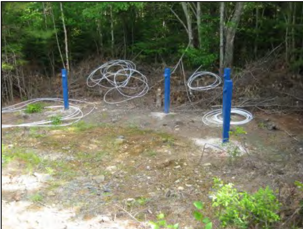
Typical cluster of monitor wells installed in various locations on and around the Site
