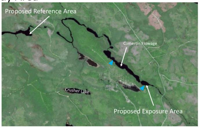
Proposed Treated Effluent Discharge Locations
