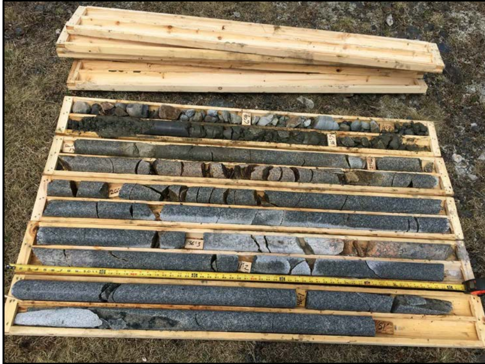
PHOTO 3 - ROCK CORES TAKEN FROM MONITORING WELL "MW02B"
