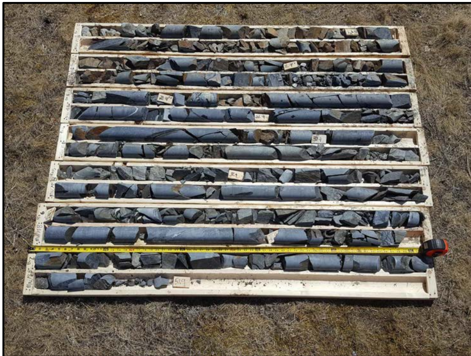
PHOTO 4 - ROCK CORES TAKEN FROM MONITORING WELL "MW18B"
