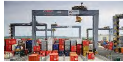
Automatic Stacking Crane (ASC)
