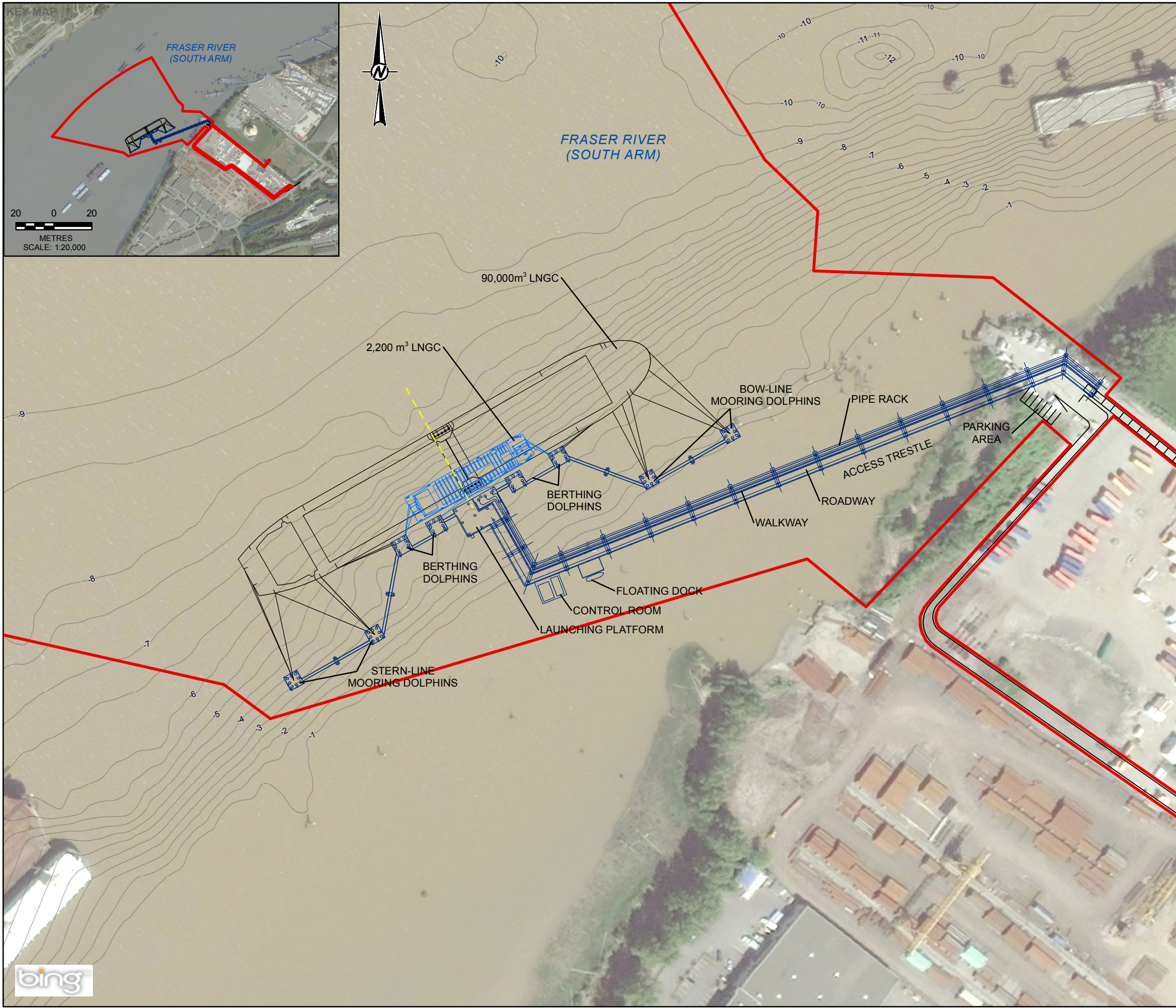
FIGURE 4 ACCESS TRESTLE AND LOADING PLATFORM DESIGN
