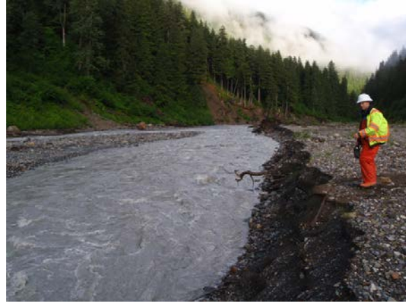
Photo 10: Looking downstream along main channel & eroding bank section in the vicinity of Stn 3+100. June 14, 2017.
