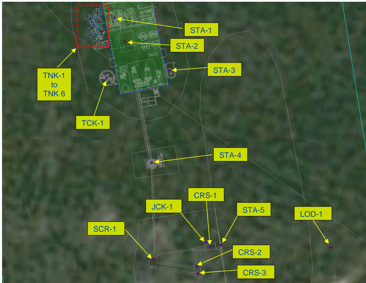
Figure 6-3 Noise Sources Location (Near Process Plant)
