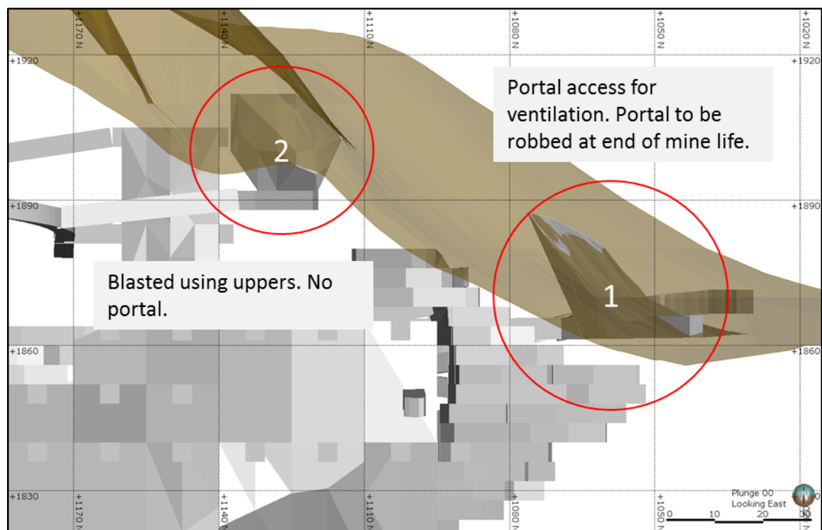
Figure 7.14: Portal near Marc zone called the lower crown (1) and the location of the upper crown (2). Gloryhole mining will be undertaken at both locations. Topography is overlain to show approximate geometry.
